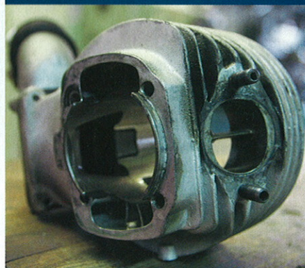
The prototype 175cc 64mm bore smallframe kit is "absolute maximum!" Look how close the studs run to both the bore and the transfer ports.
