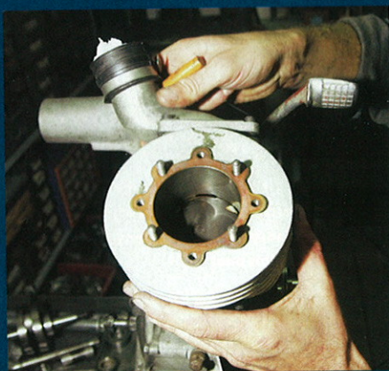
The reed valve Falc smallframe cylinders feature a reversible manifold so the carb can be used in standard position or breathing through a sidepanel cut-out. Note the eight-point head fixing on the 175cc version.
