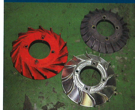
Lauro identified a problem with the fans for the popular Vespatronic and Parmakit ignitions. The orange Vespatronic fan blows well at low rpm but causes the air to cavitate (swirl around the fins rather than blowing) at high rpm resulting in insufficient cooling. The grey Parmakit one by contrast is too efficient and knocks over 3hp off the output of one of his race motors. His solution was to get a new fan CNC machined from aluminium billet that is designed to cool well without causing too much drag.
