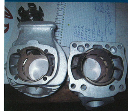
Comparing a Honda RS125 race cylinder to the 150 Falc kit. With the Vespa stud pattern it's not possible to add any more transfer port area.
