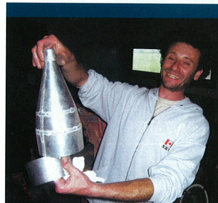
Lauro races 125cc hydroplanes. For those the exhausts are adjustable in length by foot control to widen the power band so he makes them from aluminium to save weight.
