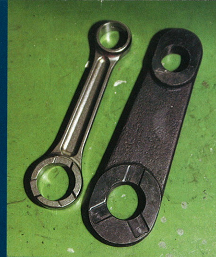
A blank forging and a finished con-rod which is tempered after machining. The Vespa rods are the same quality as the ones he uses for Grand Prix engines.
